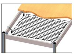
Mounting combination flush/projected: In order to prevent the possibility of the legs touching the cable grid, remove the prolongati on the user side.
