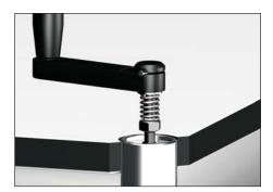
Setting the toothed wheel into final position, on the hexagon of the spindle, do not use excessive pressure. Excessive pressure will prevent from finding the correct position.
