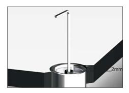
The final position of the toothed wheel is correct when it is 2 mm lower than the upper edge of the table leg. Insert the screw M3x20 and tighten with the allen key.
