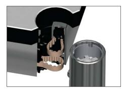
Carefully disassemble the table legs. Take care not to damage the toothed belt during transport.
