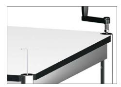
Using a 2.5 mm Allen key, loosen the screws between the toothed wheel and spindle on all table legs. To prevent the toothed belt revolving as well, check its movement by means of the crank.
