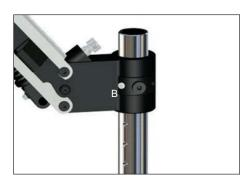
Slide the swing arm on to the frame tube and position it according to the notches. Fix adjusting collar with the thread bolt B in the notches.
