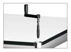
Use the crank to insert the toothed wheel into the toothed belts by turning to left and right to set in place.
