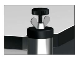
Screw the knurled screw of the pull-off tool into the toothed wheel until the stopping point is reached.
