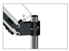
Adjust the spring tension D exactly to the weight of the flat screen (Max. 9 kg). Determine the swing range with 2 countersunk screws E on the setting collar.
