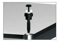
Turn the wing nut downwards until the stopping point is reached, then carefully remove the toothed wheel.
