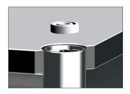
Place the table on the floor. Insert the ball bearings into the toothed wheel on all of the table legs.
