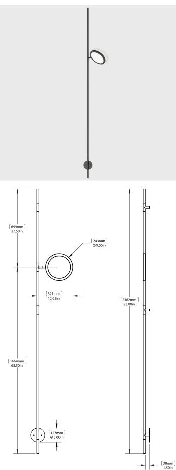
Discus is a spare and graphically compelling lighting collection. Made from modular components, the design is adaptable for spaces ranging from intimate to monumental. Dimmable LEDs cast a warm diffused light through both sides of each rotatable disc.
